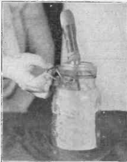
When working on your outdoor antenna, the greatest difficulty is to keep the soldering iron hot. Above we have a very clever method of avoiding this, by lining a large size preserve jar with sheet asbestos and placing the iron in the jar. (Hayden)
